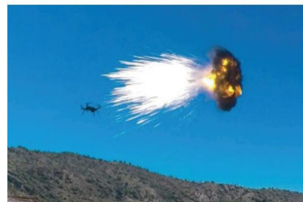
Kinetic C-UAS using airburst munition
