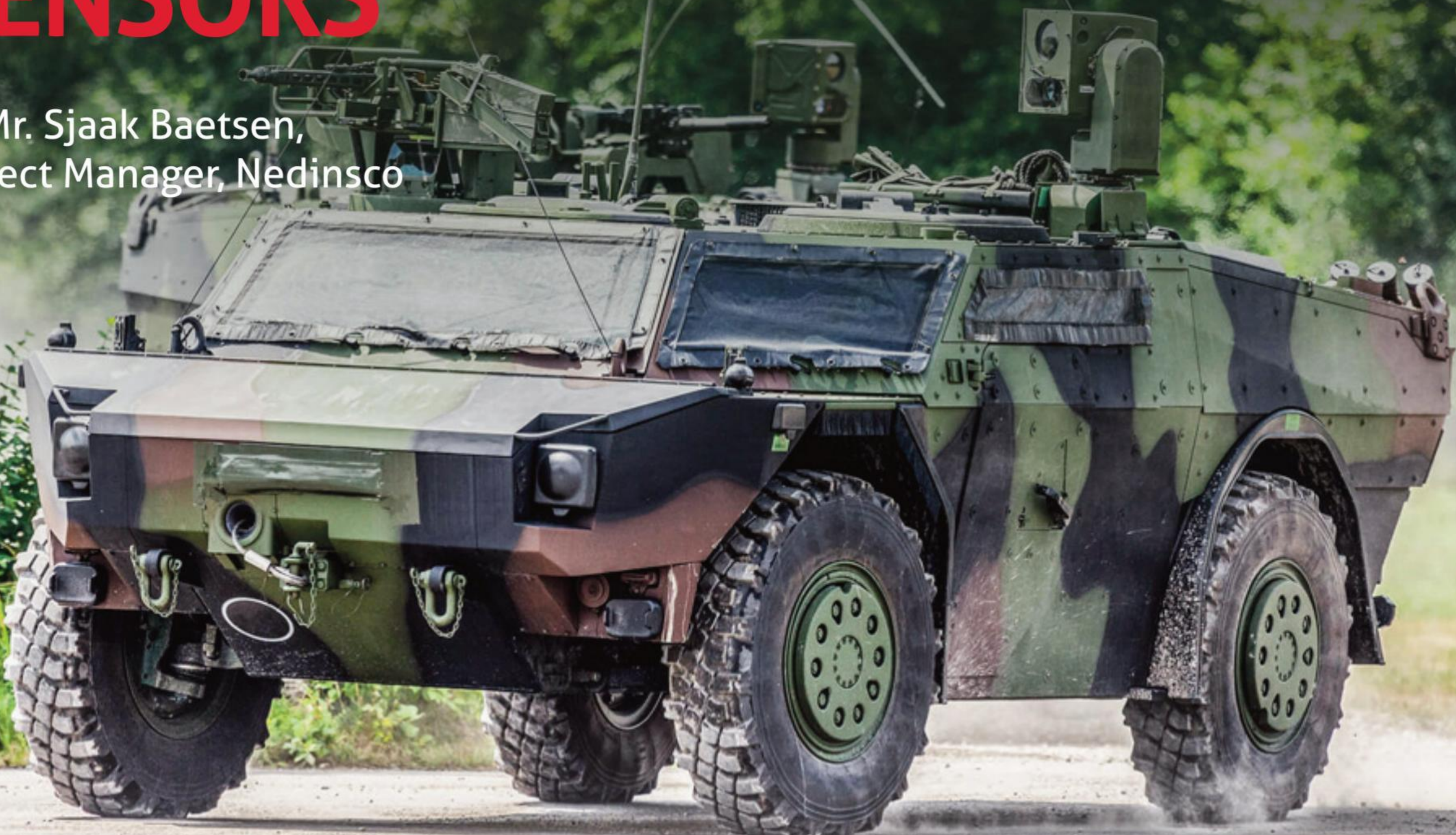
Nedinsco multi-sensor optronic units installed on an armored vehicle
