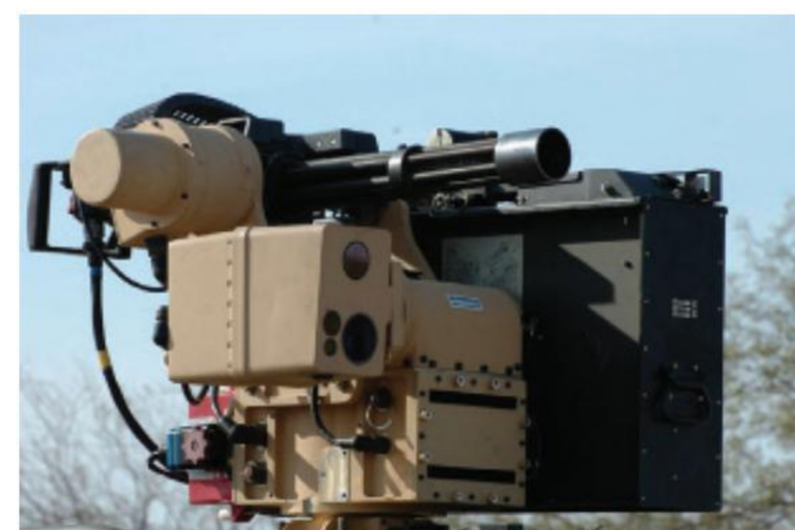
RWS fitted with Dillon Aero M134-Series Minigun
